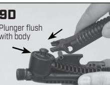
Tighten plunger clockwise until flush to top of shut-off body. Do not over-tighten or unit may not spray. Slide forks under plunger, push handle down until it snaps into place.
