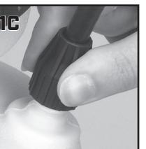
**Do:** Slide nut down over threads. Turn nut clockwise as tight as possible.
