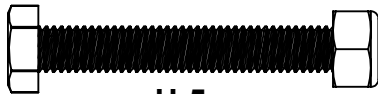
H-5 M6 X 45mm Hex Bolt Perno hexagonal M6 x 45mm Boulon hexagonal M6 x 45 mm
