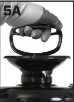
Turn handle clockwise to tighten. Push handle down, turn 1/4 turn counterclockwise to release.
